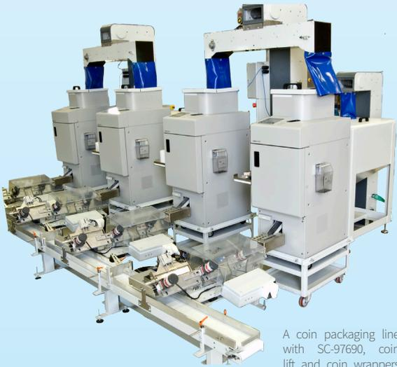
A coin packaging line with SC-97690, coin lift and coin wrappers
